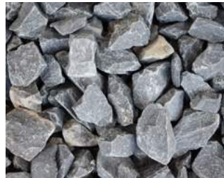
Basalt-Schotter ca. 31,5/63 mm, gebrochen
