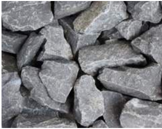
Basalt-Gabionenstein ca. 60/120 mm, gebrochen
