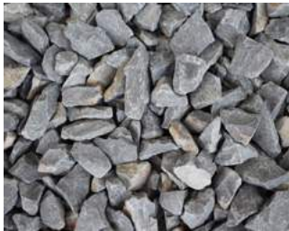
Basaltsplitt ca. 16/32 mm, gebrochen
