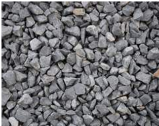
Basaltsplitt ca. 11/16 mm, gebrochen
